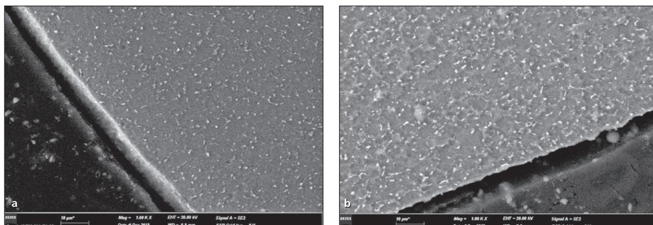
**Fig 8** Cross-section of SEM images of abutment screws. (a) Nontreated. (b) Anodic oxidation.
