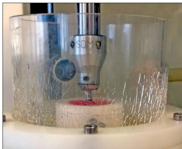
**Fig 5** Force applied in the middle of the abutment.
