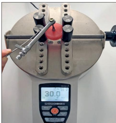
**Fig 3** Digital torque meter used to test the implant-abutment connection.
