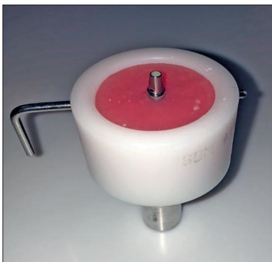
**Fig 1** Single-unit implant-abutment connection embedded in an acrylic resin model.
