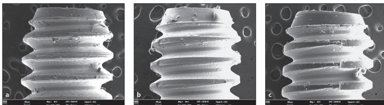
**Fig 7** SEM images of abutment screws in the thermomechanical cycling group. (a) Nontreated. (b) Anodic oxidation. (c) Diamond-like carbon coating.
