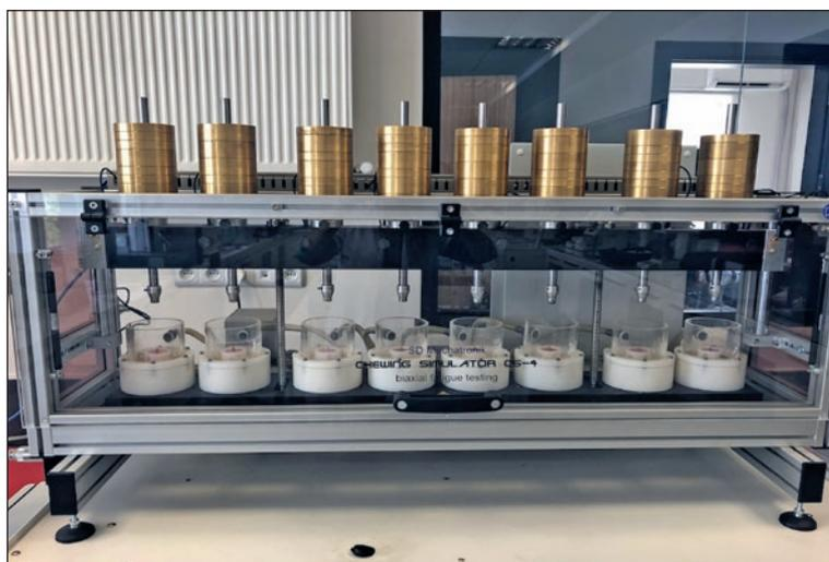
**Fig 4** Chewing simulator used for thermomechanical cycling.
