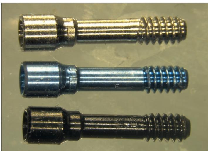
**Fig 2** Abutment screws subjected to different surface treatments in the experimental groups. From top to bottom: nontreated, anodic oxidation, and diamond-like carbon coating.
