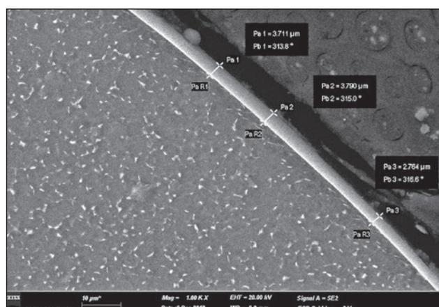
**Fig 9** Measurement of diamond-like carbon thickness.
