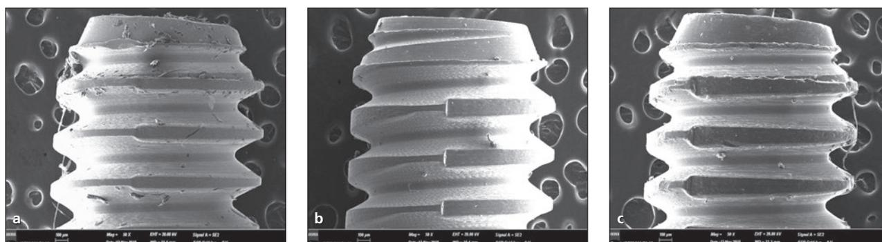
**Fig 6** SEM images of abutment screws in the non-thermomechanical cycling group. (a) Nontreated. (b) Anodic oxidation. (c) Diamond-like carbon coating.
